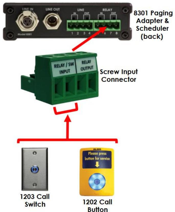
**1202 Call Button:** A pair of wires from the terminal block Relay Input on the back of the 8301 Paging Adapter & Scheduler can connect to the **centre pair** of the modular connector at the back of the Call Button.
