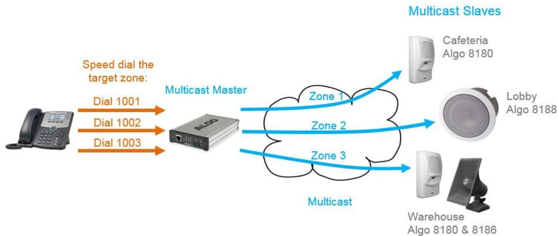
"Expanded" zones can also be enabled, allowing up to 50 zones in total. These have the same behaviours as the basic zones, but are hidden by default to simplify the interface.
