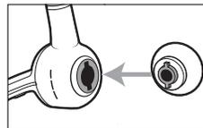
To wear the headset on your other ear, rotate the boom upwards then twist it around so the eartip is on the other side before lowering the mic boom.
